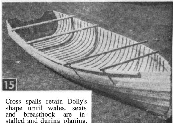
15 Cross spalls retain Dolly's shape until wales, seats and breasthook are installed and during planing.
