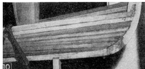
Port and starboard bottom strip planking applied around forefoot and up the stem.
