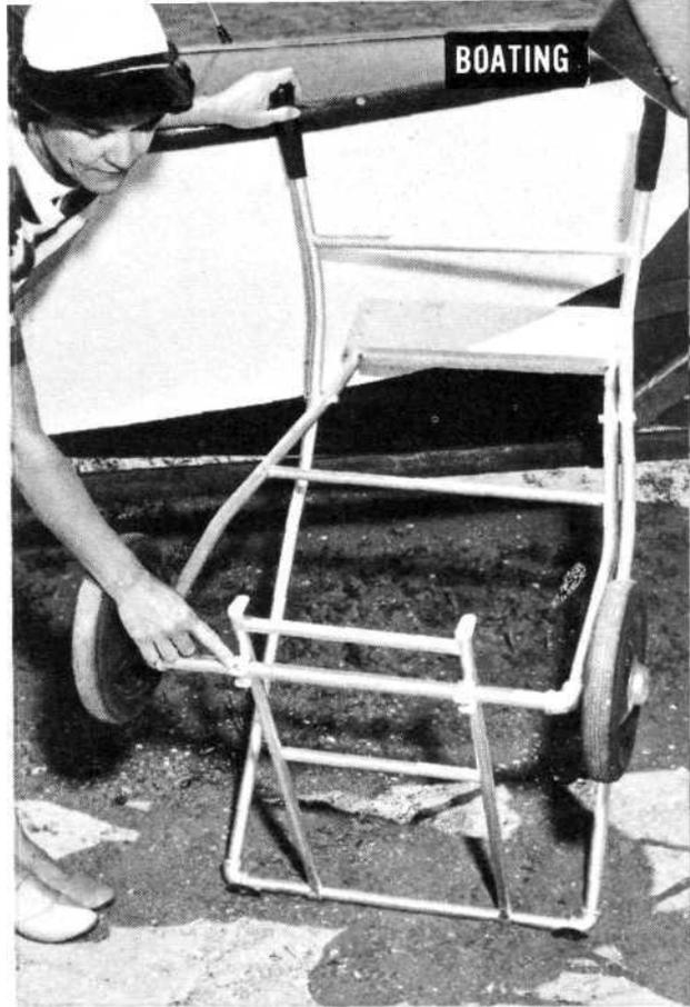
Cart is tilted up to show how single cotter pin (through U bracket) locks platform to bottom rear crosspiece.
