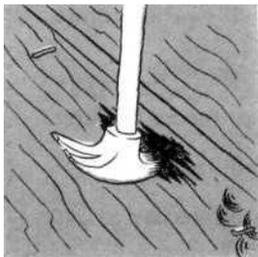
The drift will curl the point back into the wood. When you find that method doesn't work, pound the nails through, hold the drift on their heads, and bend the tips over with your hammer. If you still have trouble, remember a few hammer marks add character to your work.
